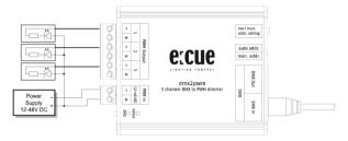
Make sure that the power supply cables are specified to carry the complete amount of current needed by the connected LED fixtures.
