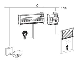
In this case, due to the fact that the roller shutter requires a certain running time to open, the light needs to be switched off with a switch-off delay so that it doesn't suddenly become dark prematurely.
