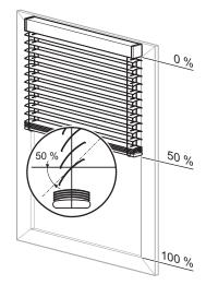
Step 2: Height running time = 24 s, upwards direction (Difference between current position 50 % and new position 30 % = 20 % of height running time) plus
