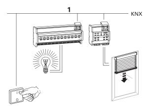
Push-button action to OFF=> telegram value "0" => light OFF and retrieve preset position 1 = open roller shutter:
