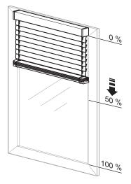
Step 3: Slat adjustment into the working position after downwards movement = **1.25 s** (Slat running time from 100 % to 50 %)
