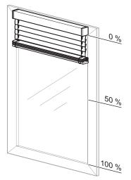
Step 2: Height running time = 60 s, downwards direction (Difference between current 0 % and new position 50 % = 50 % of height running time)
