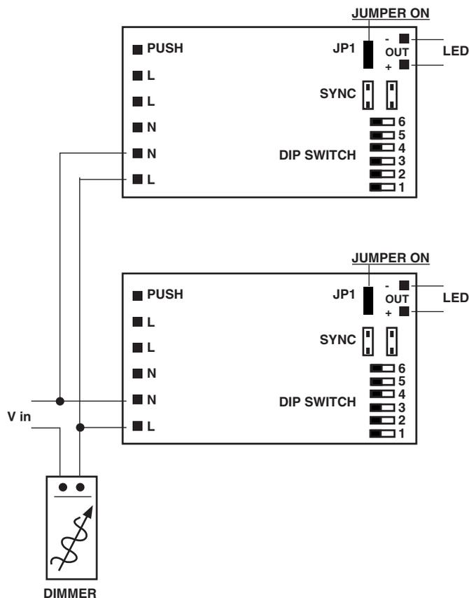
**PHASE-CUT DIMMING - To avoid flickering, keep the slaves at 100% dimming level.**
