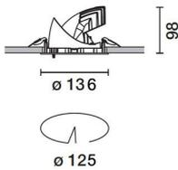
**Product code**MU43: extractable, adjustable, recessed LED luminaire - electronic control gear included **Attention! Code no longer in production****Technical description**
