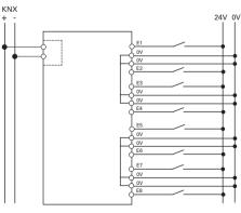
The 0 V conductors must be connected to the i device. Inputs E1 to E4 have a common potential (4 x 0 V, top row) and inputs E5 to E8 have a common potential (4 x 0 V, bottom row).
