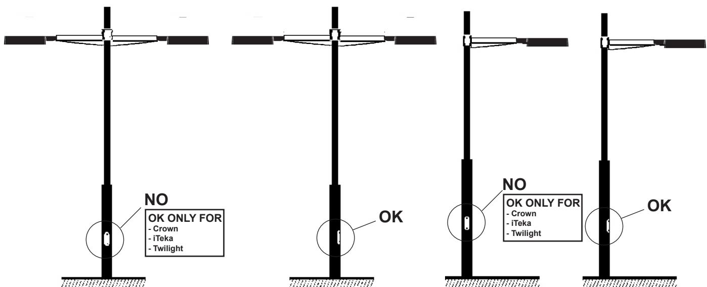
TIPO DI INSTALLAZIONE DEL PALO - POLE INSTALLATION TYPE - TYPE D'INSTALLATION DU MÂT - INSTALLATIONSTYP DES MASTS
